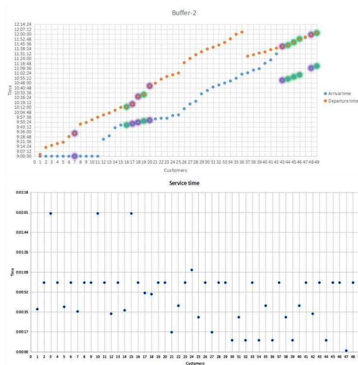
**Figure 4.** Arrival and departure times together with service times in Server-2 for Buffer-2. A point with green shadow represents a customer moving from Buffer-1 to Buffer-2 and a point with purple shadow represents a customer moving from Buffer-3 to Buffer-2 for service.
